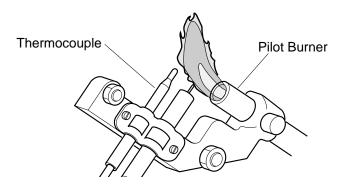
Figure 20 - Incorrect Pilot Flame Pattern
